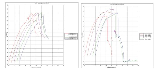
Conclusion: No failure of the posts at 23°C but also at -40°C. The part is still very flexible and therefore there is little or no risk of failure of the posts, even at -40°C t and when the part returns to room temperature it tends to return to its original shape.
